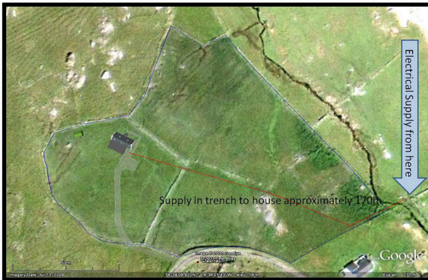
Figure 8: The Electrical supply will be in a trench from an existing transformer
